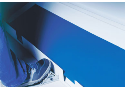
Foot lever for adjusting the parts chute: Sorting to the front and the rear
