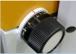
Fast blade clearance adjustment for burr-free cuts
